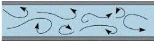
Gambar II.2 Aliran Turbulen
