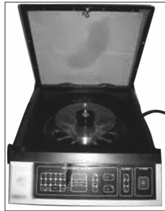
Figure 11.1: Cytocentrifuge or Cytospin
