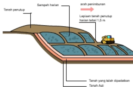
Gambar 2.2 Metode Controlled Landfill (Sumber : Nurul, 2013)
