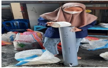
Gambar 13. Proses pengisian media filtrasi
