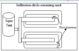
Figure 1 Design of Tripikon Infiltration
