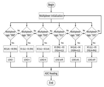
Fig 3. The Flowchart of the Multiplexers
