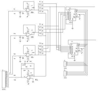
Fig 4. Circuit of Selection leads with multiplexers
