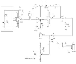
Fig 5. Circuit of Instrumentation
