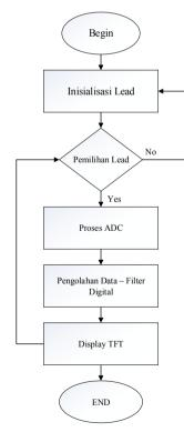
Fig 2. The flowchart of development of a low-cost and efficient ecg devices with IIR digital filter design
