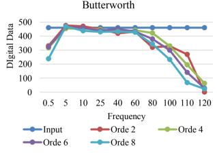
Fig 7. Digital Filter using Butterworth Type
