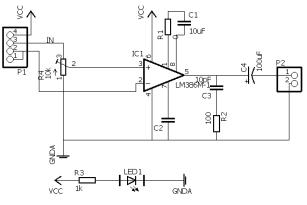
Fig. 6. Amplifier LM386 with gain 200
