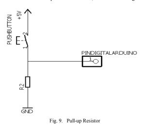
In Fig. 9 The pull-up resistor circuit serves to address the floating conditions of the float is a volatile condition between high and low. This circuit is required when providing digital input to the Arduino. The pull-up resistor circuit is used for the
