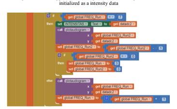
Fig. 15. The Mit App Inventor 2 Program when receiving B record is
