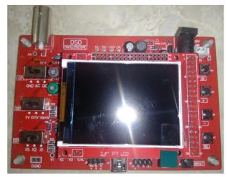
Fig. 11. DSO138 Digital Oscilloscope
