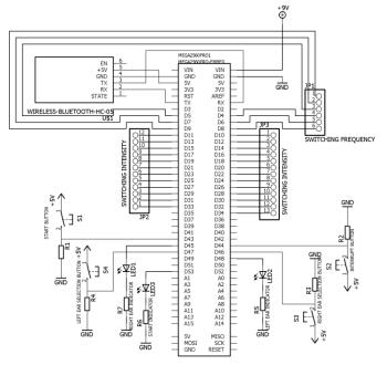
Fig. 10. Mikrokontroller Arduino ATmega2560 Pro Mini circuit
