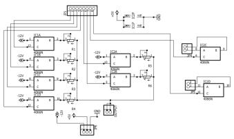
Fig. 3. Frequency Switching with CD4066
