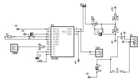
Fig. 4. Generator Frekuensi 250-8000Hz with XR2206
