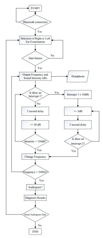
Fig. 2. The Flowchart of Automatic Pure Tone Audiometer
