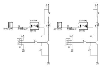
Fig. 8. Right or left Headphone selection circuit with Solid State Relay
