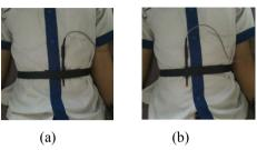
Fig. 10. Sensor placement to measured the respiration (a) left (b) right side
