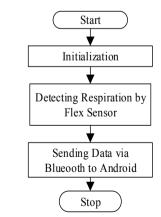
Fig. 2. The flowchart of the arduino program
