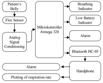
Fig. 1. The diagram block of the apnea monitor
