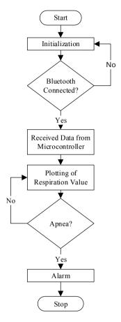
Fig. 3. The flowchart of the android program
